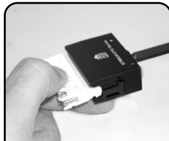
**8** Insert a connecting block (P/N: S210C-4) into the head of the Siemon termination tool.
