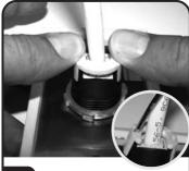
Install retention clip, seat in place as shown. To remove clip, insert a small bladed screw driver as shown and pry gently.
