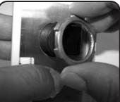
Place the panel nut over the flange and tighten to 1.69-2.26N-m (15-20 in-lbs). The teeth on the nut should face toward the faceplate.
