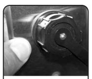
Secure the dust cap in position on the outlet and rotate ¼ turn clockwise to lock in place.
