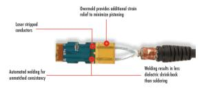
SFP+ passive copper cables contain EEPROMs within the connector back shell that have I2C ports. These cables may also be referred to as DAC or "direct attached copper" cables. An EEPROM is an "Electrically Erasable Programmable Read-Only Memory" chip that is programmed at the factory with specific information about the cable assembly.
