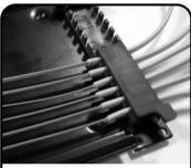
After loading is complete, insert rubber cover over holder and jacket.
