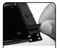
When using unjacketed ribbon fiber, insert provided grommets into the holder slots as shown.
