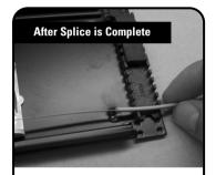
When using oval jacketed ribbon, lay directly into ribbon jacket holder.
