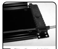
Ribbon fiber can be laid into the installed grommets.
