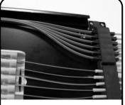
After loading is complete, insert rubber cover over holder and fiber.
