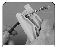
Strip back as much of the cable jacket as is needed [approximately 40mm (1.5 in.)] using the Siemon AllPrep™ tool (P/N: CPT-RGTP) or equivalent.
