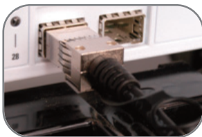
Figure 1. Installing an SFP+ Module
