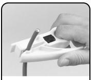
Using a Siemon ALLPREP™ (P/N: CPT-RGTP) tool or equivalent, remove approximately 38mm (1.5 in.) of sheathing.
