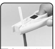
Remove the inner jacket leaving 6mm (0.25 in.) of inner jacket.
