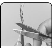
Cut the rip cord as close to the jacket as possible. Fan pairs into proper color code (see next frame).
