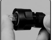
Insert the modular plug into the plug housing. Align the latch with the LATCH slot, depress latch, and insert plug into plug housing until it bottoms out.
