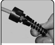
Place plug housing over the Industrial cable as shown, flex nut may need to be loosened.
