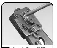
Using the Siemon PT-908 crimp tool or equivalent, terminate the modular plug to the cable.
