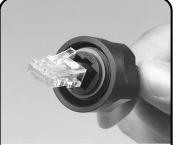
Slide the plug housing up the cable and align with the modular plug.
