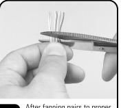
After fanning pairs to proper color code, hold the pairs close to the jacket and trim conductors leaving 12mm (0.5 in.) extending from the form
