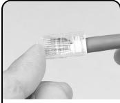
Place modular plug over wire ends being sure to maintain color code. Insure that the pairs are inserted all the way into the modular plug including the inner jacket. The inner jacket should be directly under the plug's strain relief tab.
